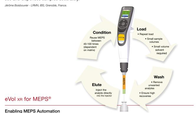
MEPS® is Micro Extraction by Packed Sorbent, the miniaturization of conventional SPE packed bed devices from milliliter bed volumes to microliter volumes. The MEPS approach to sample preparation is suitable for reversed phase, normal phase, mixed mode or ion exchange chemistries.
